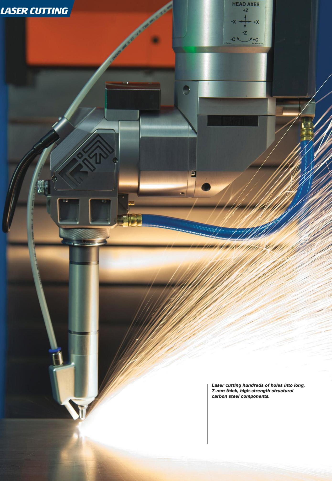
*Laser cutting hundreds of holes into long, 7-mm thick, high-strength structural carbon steel components.*
