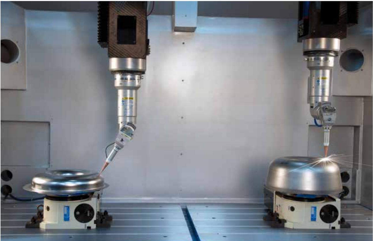
Two 6-axis machines consisting of three linear axes, two rotary axes of the BeamDirector(R), and fully integrated rotary axis for workpiece indexing and contouring.
