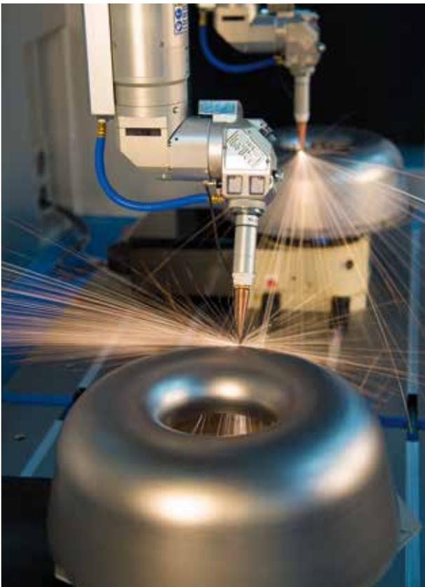
LASERDYNE 606D can be used to process completely different parts or perform different operations in each of the workstations.
