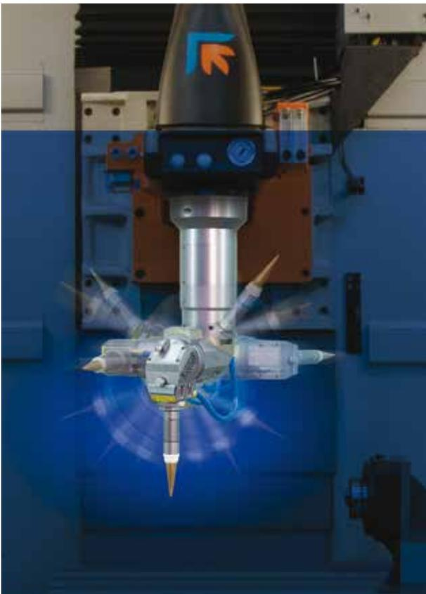
The LASERDYNE BeamDirector provides 900 degrees of rotary motion and 300 degrees of tilt motion.
